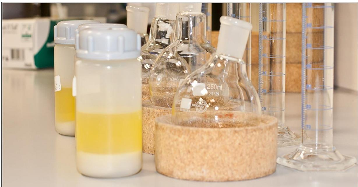
**Figure 11: Sample material following the first chemical extraction, ready for clean-up steps.**
