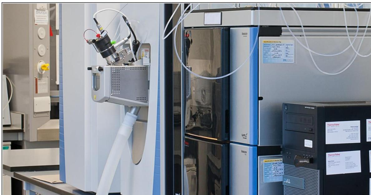
**Figure 15: State-of-the-art advanced facilities are available in the Pesticide Control Laboratory such as accurate, high resolution mass spectroscopy.**
