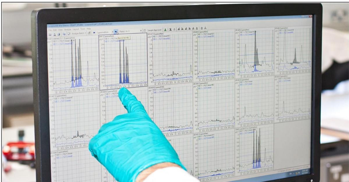
**Figure 13: Sample chromatograms being compared with pesticide standards.**
