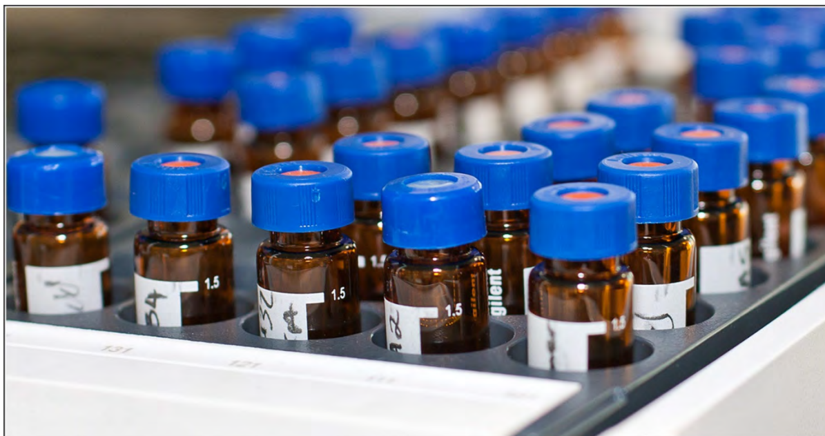
Figure 13: Glass vials containing samples for automated injection onto analytical equipment.
