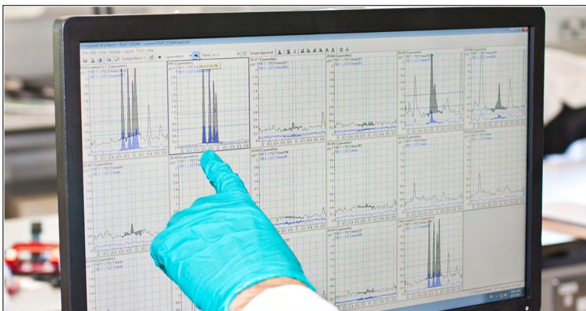
Figure 14: Sample chromatograms being compared with pesticide standards.
