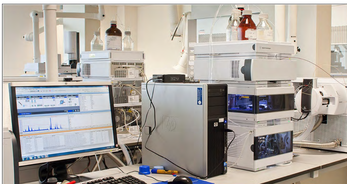
Figure 5: Pesticide Control Laboratory with liquid chromatographic systems for sample analysis.
