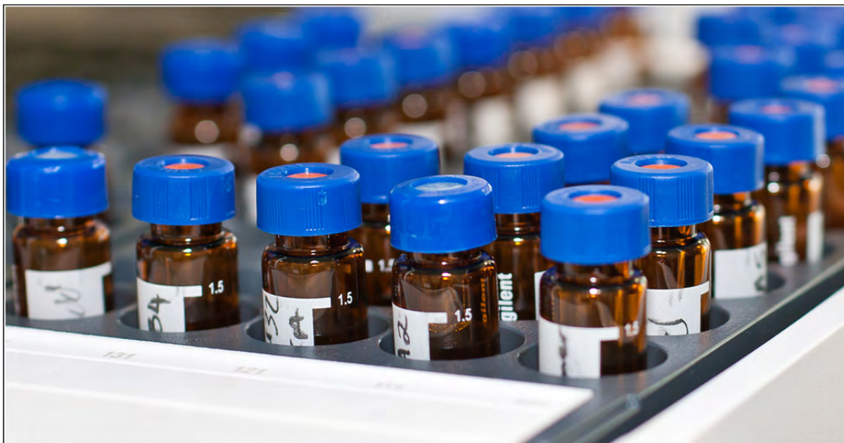
Figure 10: Glass vials containing samples for automated injection onto analytical equipment.
