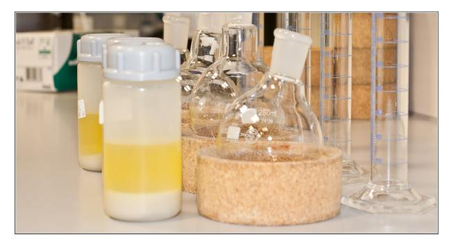
Figure 11: Sample material following the first chemical extraction, ready for clean-up steps.
