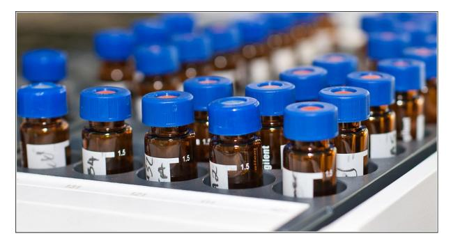
Figure 12: Glass vials containing samples for automated injection onto analytical equipment.
