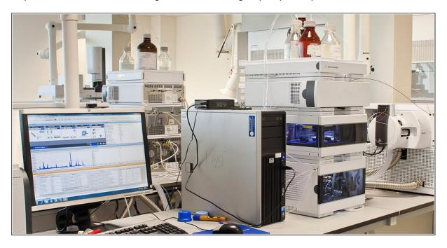
Figure 5: Pesticide Control Laboratory with liquid chromatographic systems for sample analysis.
