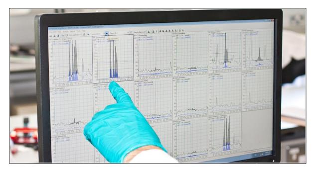
Figure 13: Sample chromatograms being compared with pesticide standards.
