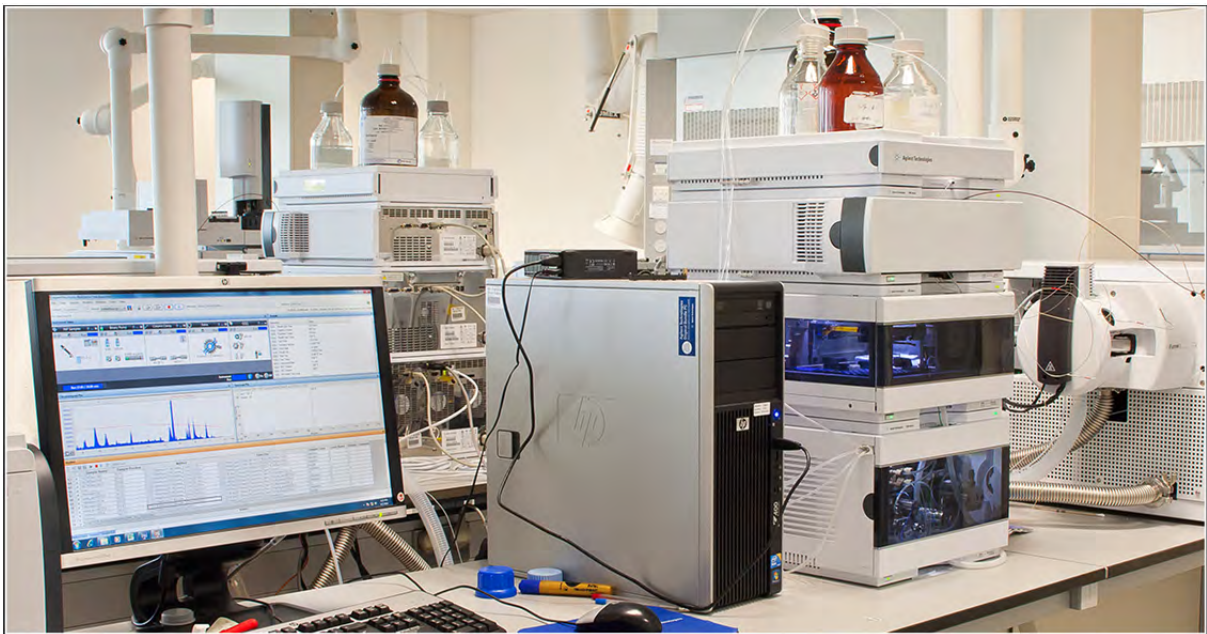
Figure 2: Pesticide Control Laboratory with liquid chromatographic systems for sample analysis.
