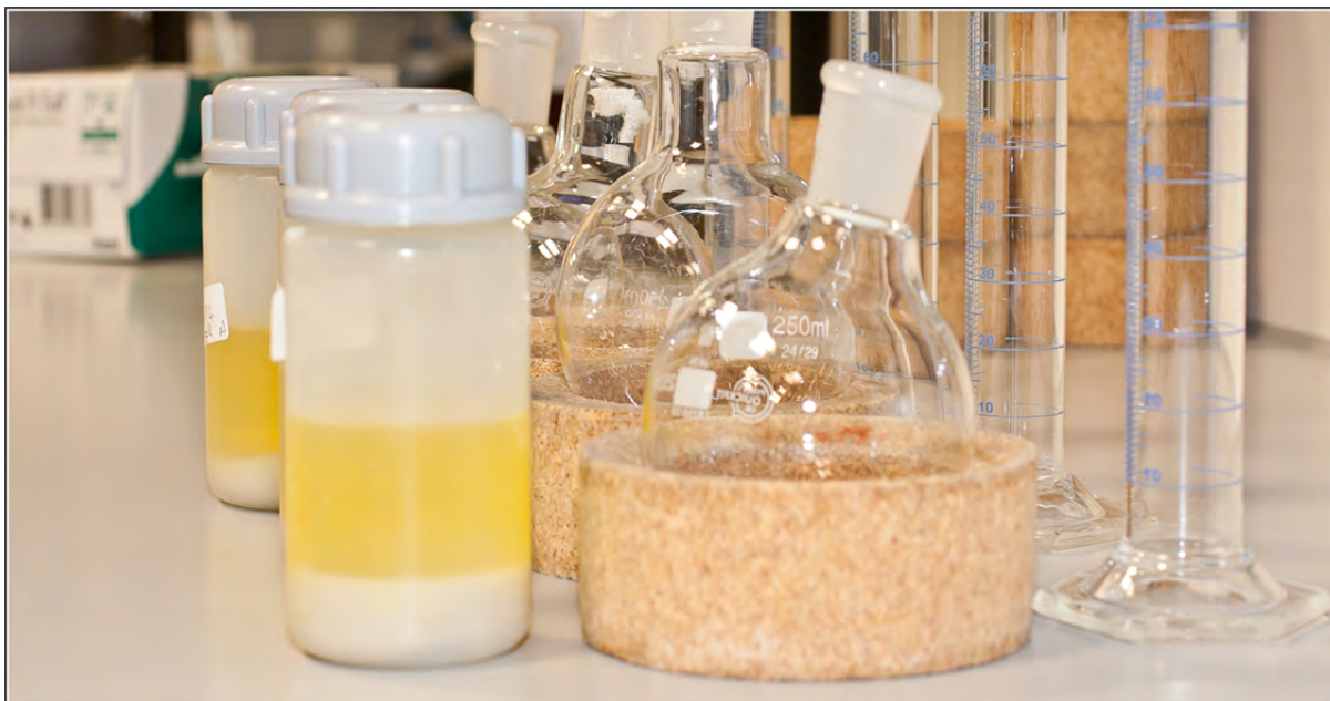
Figure 9: Sample material following the first chemical extraction, ready for clean-up steps.
